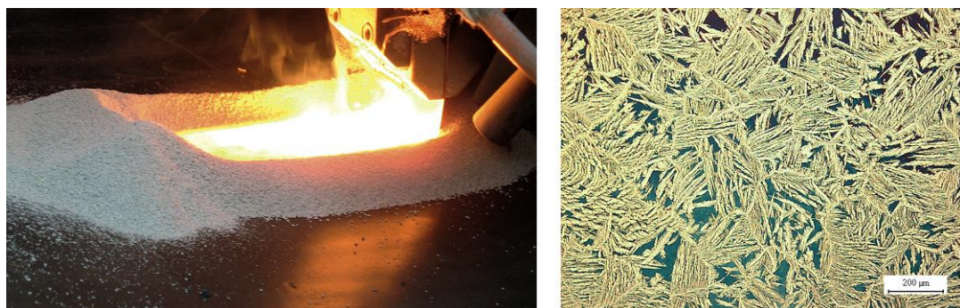
Fig. 2. Microstructure of 22%Cr duplex cladding layer (right) on mild steel. The cladding was deposited with electroslag strip cladding (left) in one layer using a 60 mm wide strip consumables with a linear energy input of approximately 11 kJ/mm. An appropriate ferrite/austenite balance was achieved and the weld metal was free from intermetallics.
