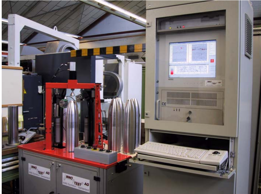
Fig 8.9.1.1: EMAT shell test system with test mechanics, service panel and electronics rack
