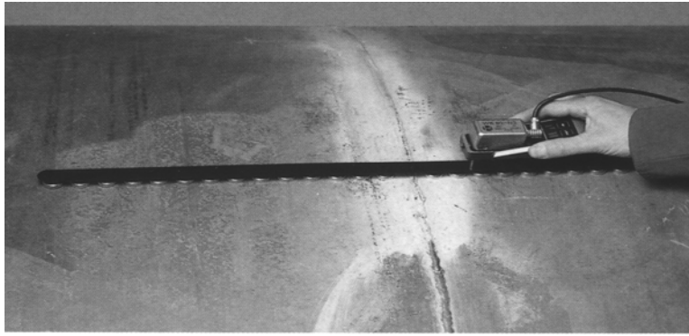
Fig 3.2.2: Simple manipulation set-up with one probe
