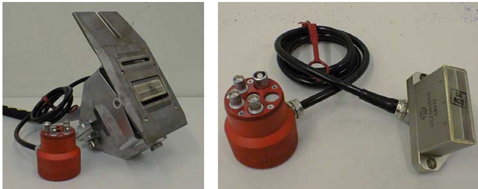
Fig 8.3.2: TR-probe in the holder (left), apart from the holder (right)
