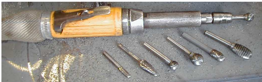
Fig. 3.1 Pneumatic grinder and burrs
