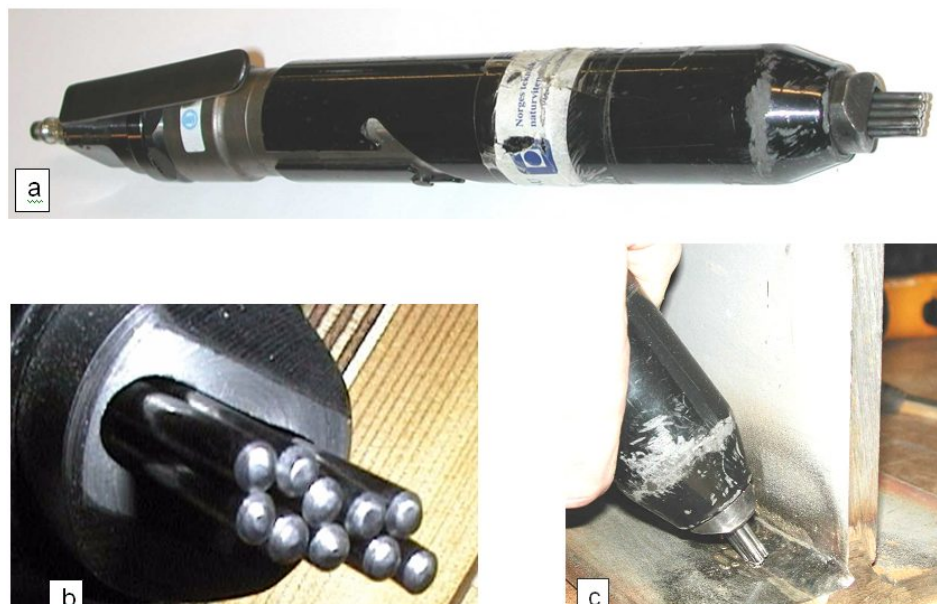
Fig. 6.1 Needle peening equipment and operation.
