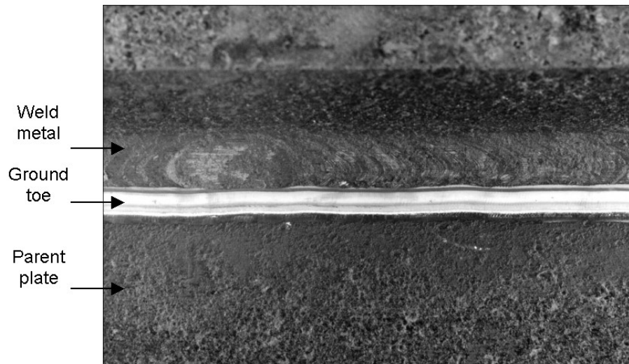
(a) Correctly ground weld toe
