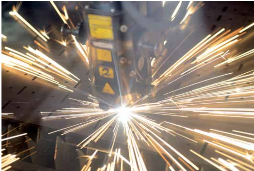
4,4kW CO 2 Bystar cutting thick sheet.
