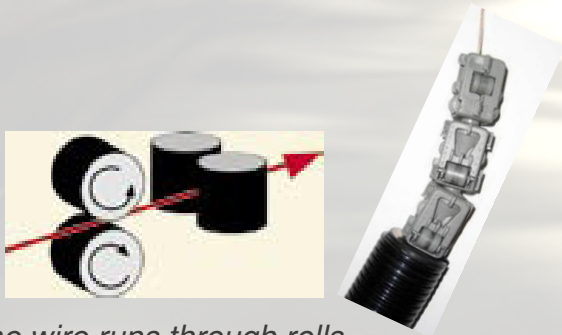
The wire runs through rolls which are shifted by 90°.
