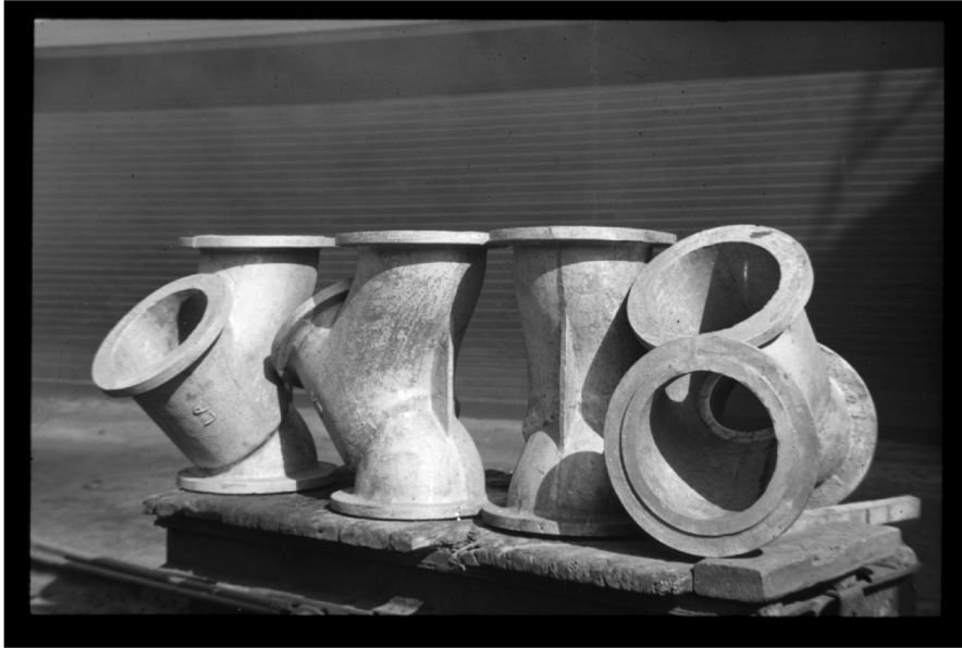
Cast valve bodies of 453S for sulfite industry
