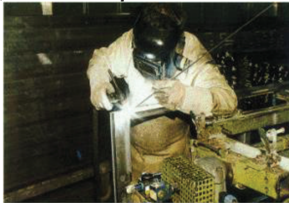
Figure 10-2: TIG welding, a process with low welding fume emission [Source: Spiegel-Ciobanu, BGI 593 Ed. 2008]
