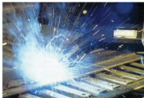
Figure 10-15a: Torch-integrated extractor out of operation
