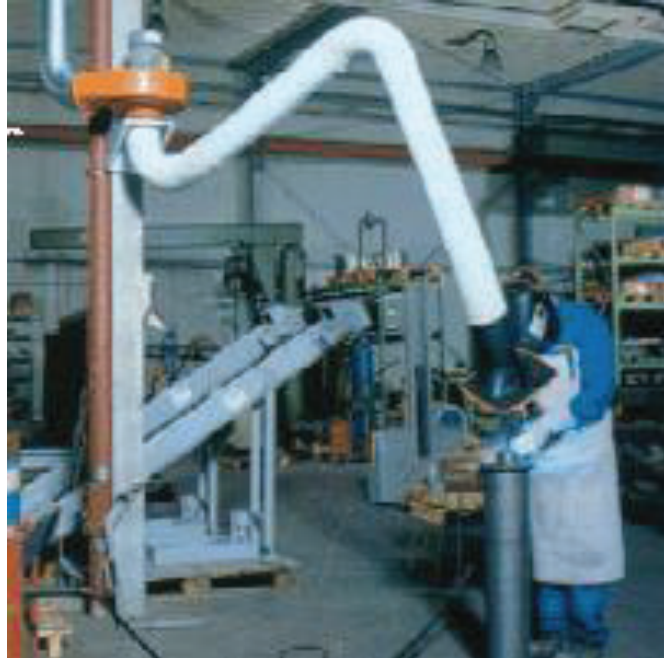
Figure 10-9: Gas-shielded metal arc welding (MIG/MAG) with extractor [Source: Fa. KEMPER]
