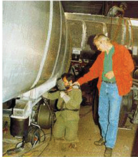
Figure 6-3: Measurement of airborne particles with a personal dust collector (PAS) and check for gaseous hazardous substances by means of detector tubes [Source: Spiegel-Ciobanu, BGI 593 Ed. 2008, Messtechnik NMBG]
