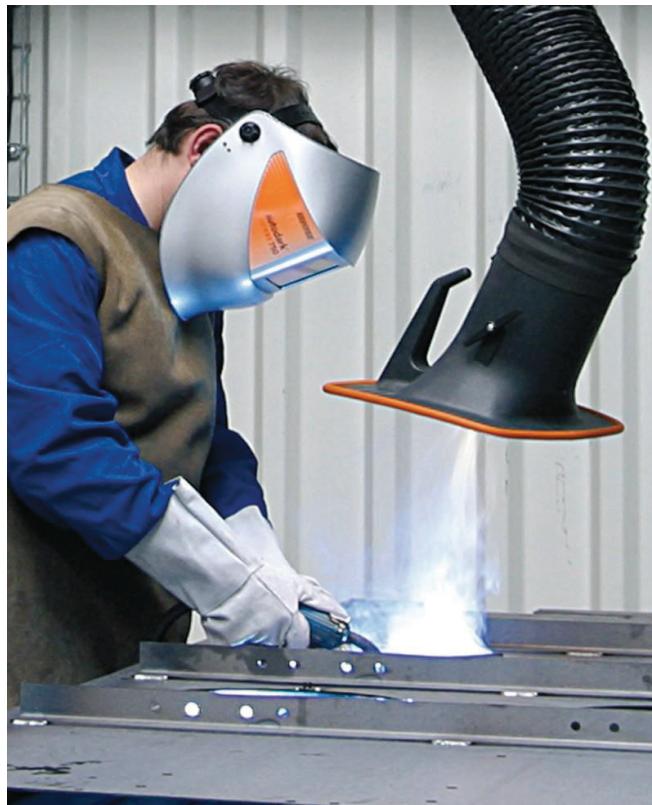
Figure 10-9: Gas-shielded metal arc welding (MIG/MAG) with extractor [Source: Fa. KEMPER]
