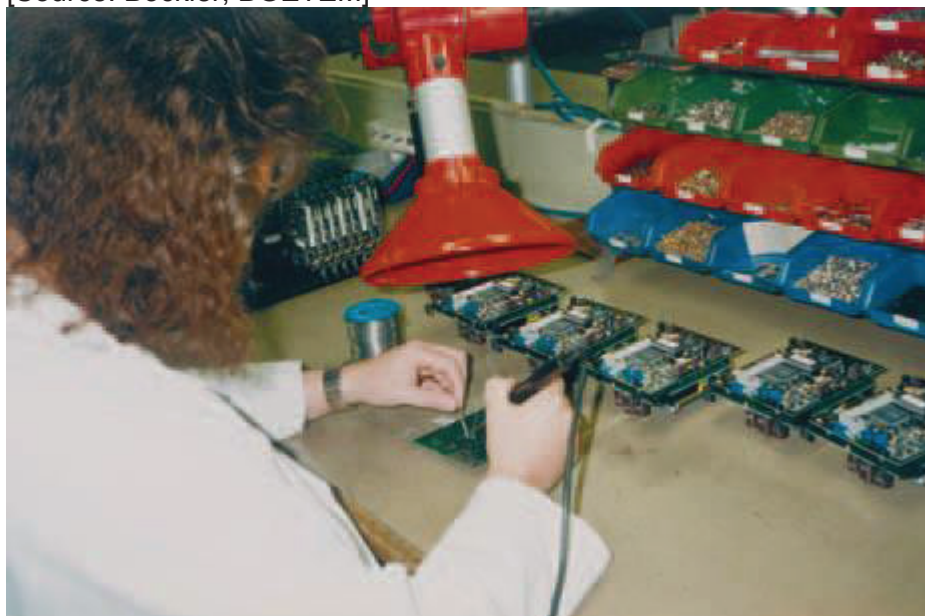
Figure 3-4: soldering workplace with extraction [Source: Böckler, BGETEM]
