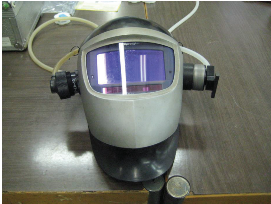
Figure 6-10: Welder's safety helmet with integrated sampling heads PGP-EA and GSP for simultaneous sampling [Source: Messtechnik BHGM/Fiegehehn]
