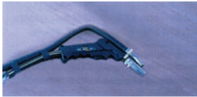
Figure 10-11: Capture element fixed to the torch
