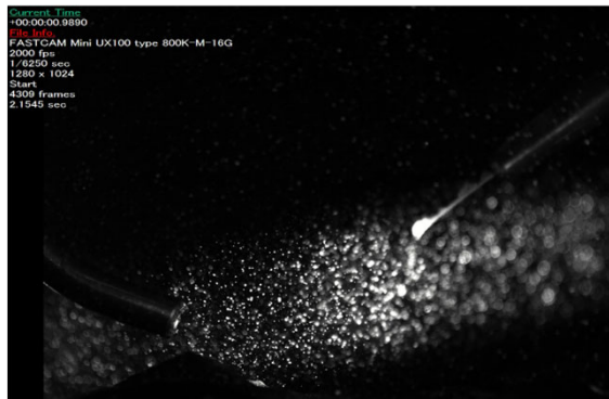
Nozzle gas flow: Visualize by bubble generator
