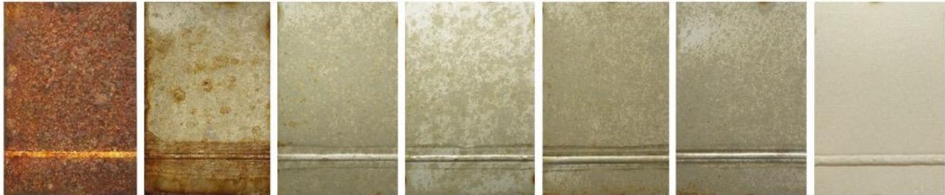
Moda 410L/4003 Moda 430/4016 Core 304L/4307 Supra 316L/4404 Forta LDX 2101 Forta DX 2304 Forta DX 2205
